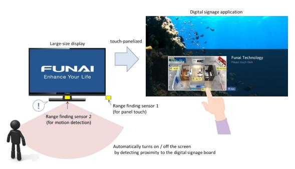
Figure 3. Application of range finding sensors to the digital signage
