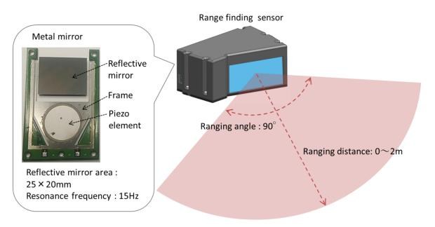
Figure 2. Function of a range finding sensor
