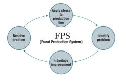
This system applies stress to the production line, such as reducing the number of operators and increasing the speed of the conveyor belt, until conditions are created such that the production line stops. The FPS creates these conditions to analyze what causes the line to stop, then improves on those conditions that caused the failure. By repeating this cycle, we hopes to realize continuous improvements to productivity.
